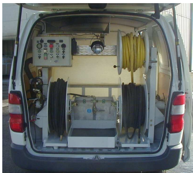
1 or 2 hydraulic hose reels Capacity 80 m of 3/8" HP hose + water filling reel
