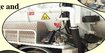
EX-protected control panels and electric components (24V plug, work lights...)
