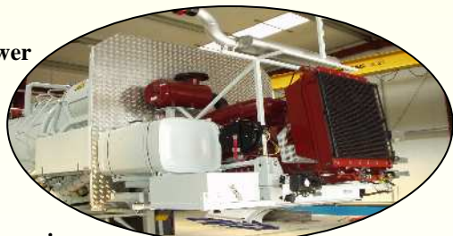
The auxiliary engine can be in conformity with the danger zone 1 or 2 and certified by INERIS
