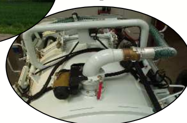
Suction arm mounted on the hose reel, fitted with isolating valve and special suction hose (for products with flash point \geq 61^{\circ}\text{C} )
