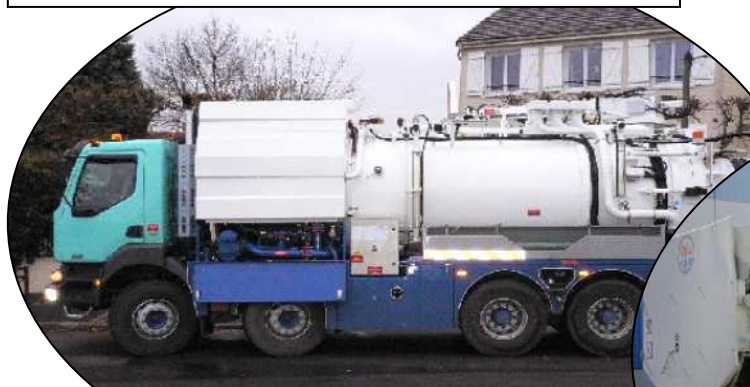
RVI KERAX 370 DCI 8X4 PHP P 2+45 (348 l / 190/205 bars) PAV : SIHI SL300
