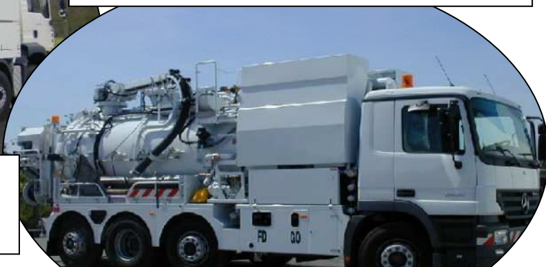
MERCEDES ACTROS J3236 NLG 8X2/6 PHP P 3-45 P60 (348 l / 190/205 bars) PAV : DELTA 3000
