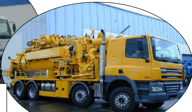
DAF FAD 82 380 8X4 PHP P 3-45 P65 (408 l / 155/175 bars) PAV : ALPHA 40+
